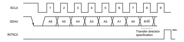
**Note** When data other than base address or extended code is received during slave operation, INTIIC0 is not generated.
