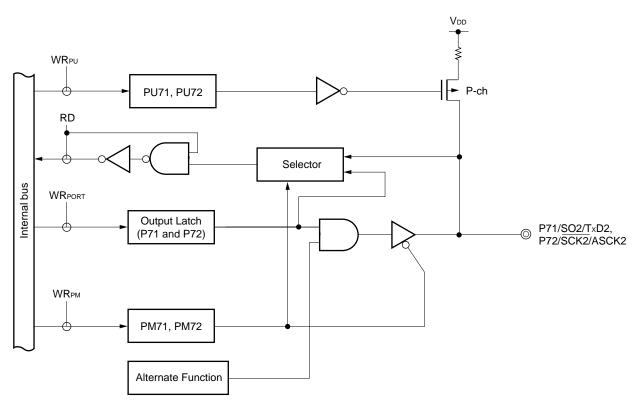
Figure 5-12. Block Diagram of P71 and P72
