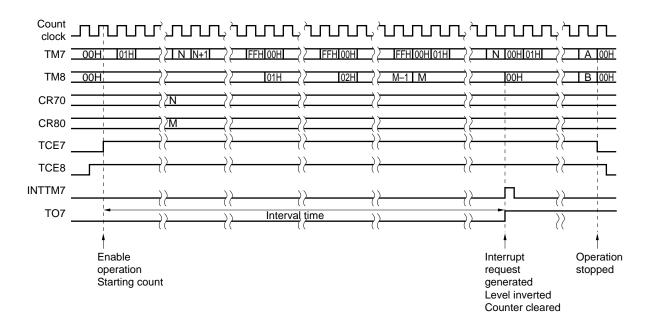
Figure 11-10. Cascade Connection Mode with 16-Bit Resolution
