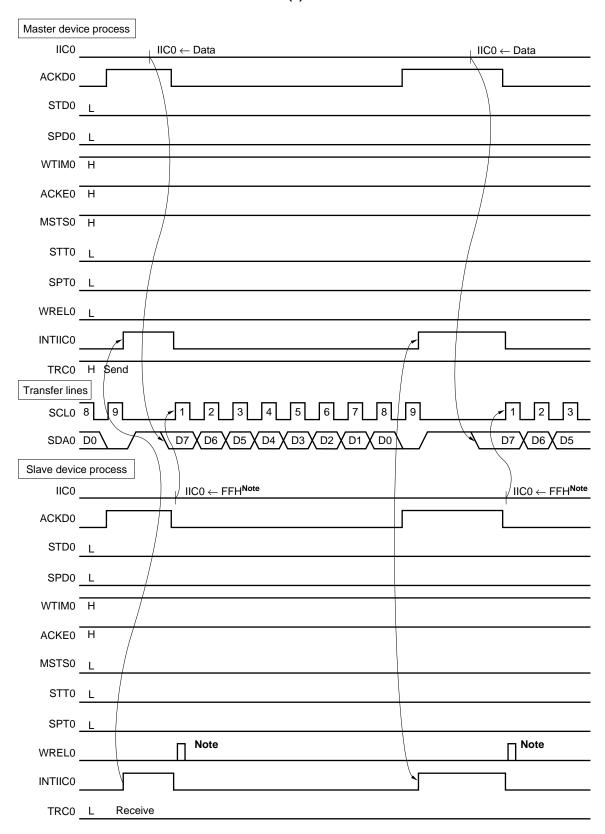
$\textbf{Note} \ \ \text{Release the slave wait by either IIC0} \leftarrow \text{FFH or setting WREL0}.$
