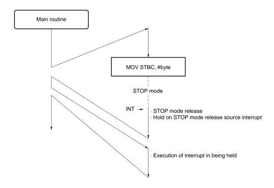
(4) STOP mode during interrupt processing routine whose priority is lower than release source interrupt
