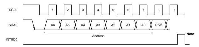
**Note** When data other than base address or extended code was received during slave operation, INTIIC0 is not generated.
