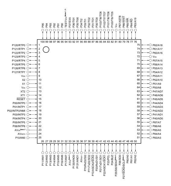
Notes 1. Connect the TEST/VPP pin directly to Vss.
