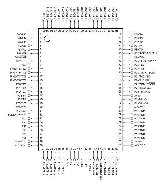
Notes 1. Connect the TEST pin directly to Vss.
