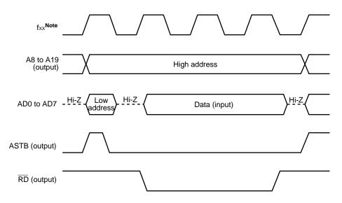
Figure 24-15. Read Timing by Access Wait Function (2/2)
