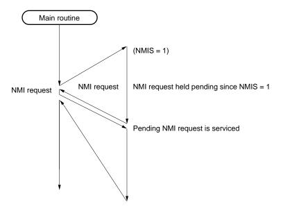
(b) When a watchdog timer interrupt request is generated during NMI service program execution (when the watchdog timer interrupt priority is higher (when WDT4 in the WDM = 1))
