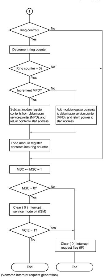
Figure 23-30. Macro Service Data Transfer Processing Flow (Type C) (2/2)
