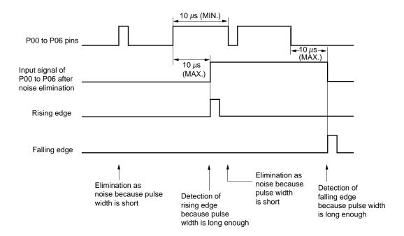
Figure 22-2. Edge Detection of P00 to P06 Pins
