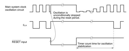
Figure 26-1. Oscillation of Main System Clock in Reset Period
