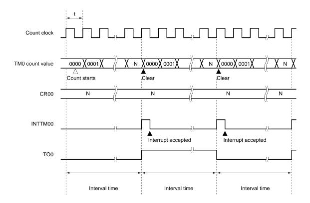
**Remark** Interval time =  $(N+1) \times t$ : N = 0001H to FFFFH
