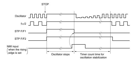
Figure 25-7. Releasing STOP Mode by NMI Input
