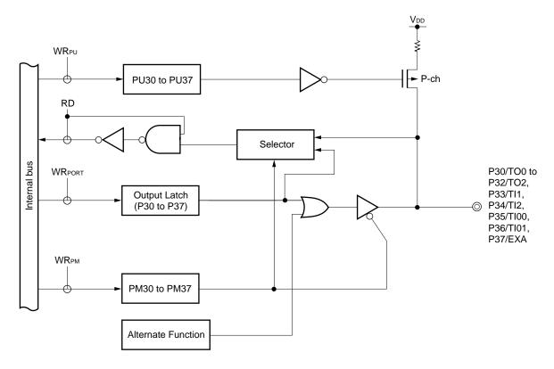
PU: Pull-up resistor option register
