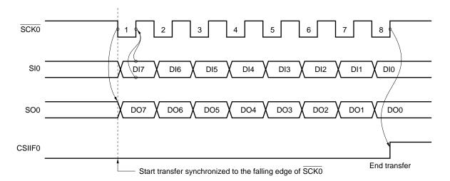
Figure 18-5. 3-Wire Serial I/O Mode Timing
