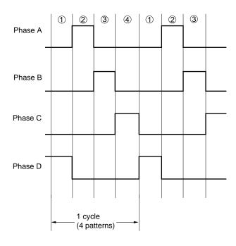
Figure 23-35. 1-2-Phase Excitation of 4-Phase Stepping Motor
