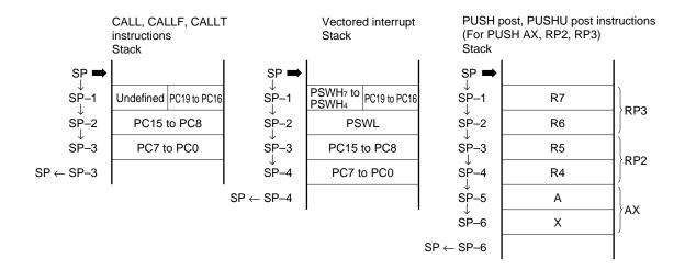
Figure 3-9. Data Restored from Stack
