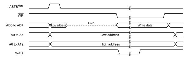
Figure 24-13. Read Modify Write Timing for External Memory in Separate Bus Mode
