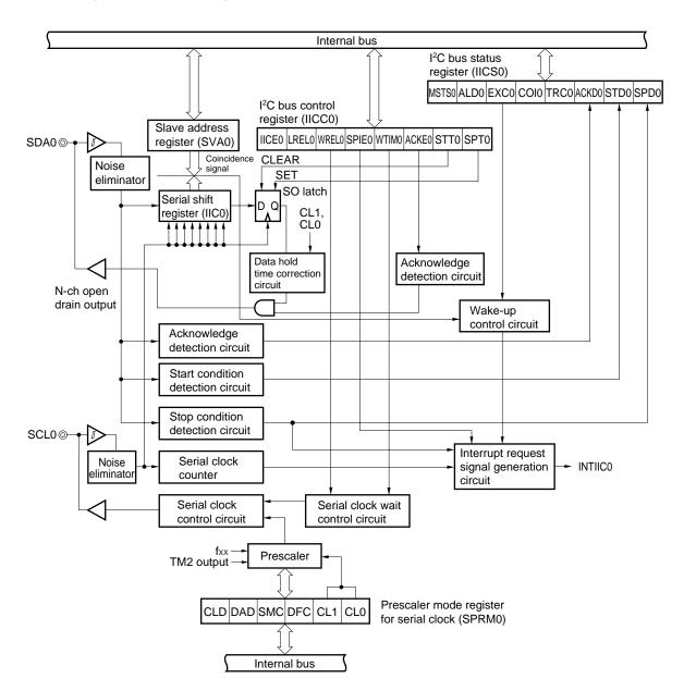
Figure 19-2. Block Diagram of Clock-synchronized Serial Interface (I<sup>2</sup>C Bus Mode)
