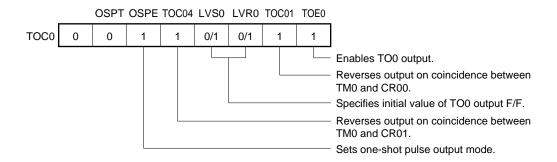
**Remark** 0/1: When these bits are reset to 0 or set to 1, the other functions can be used along with the one-shot pulse output function. For details, refer to **Figures 8-2**, **8-3**, and **8-4**.
