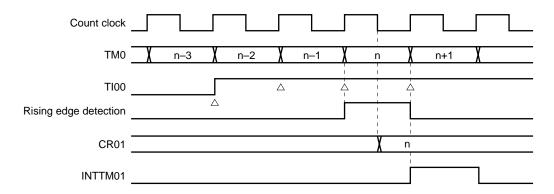
Figure 8-15. Timing of Pulse Width Measurement with Free Running Counter (with both edges specified)
