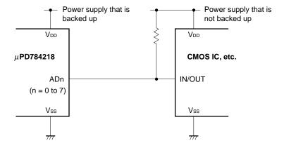
Figure 25-10. Example of Handling Address/Data Bus
