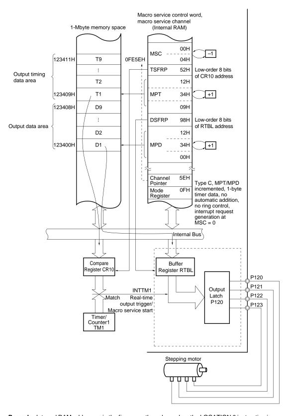
Figure 23-32. Stepping Motor Open Loop Control by Real-Time Output Port
