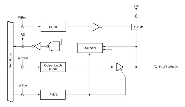
PU: Pull-up resistor option register
