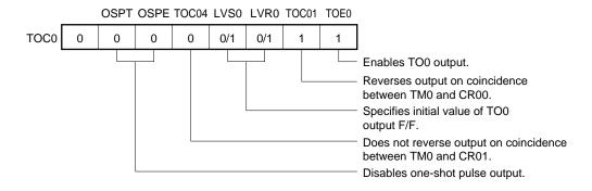
**Remark** 0/1: When these bits are reset to 0 or set to 1, the other functions can be used along with the square wave output function. For details, refer to **Figures 8-2**, **8-3**, and **8-4**.
