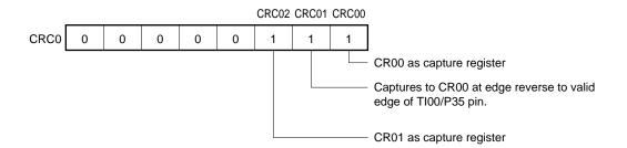
**Remark** 0/1: When these bits are reset to 0 or set to 1, the other functions can be used along with the pulse width measurement function. For details, refer to **Figures 8-2** and **8-3**.
