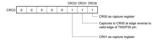
**Remark** 0/1: When these bits are reset to 0 or set to 1, the other functions can be used along with the pulse width measurement function. For details, refer to **Figures 8-2** and **8-3**.
