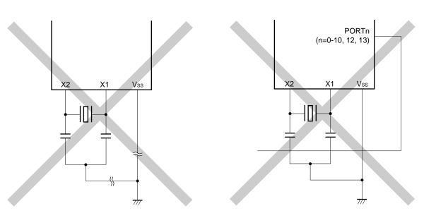
**Remark** When using a subsystem clock, replace X1 and X2 with XT1 and XT2, respectively. Also, insert resistors in series on the XT2 side.
