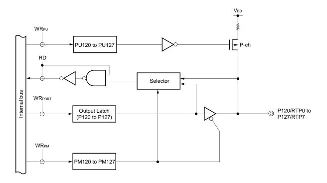
PU: Pull-up resistor option register
