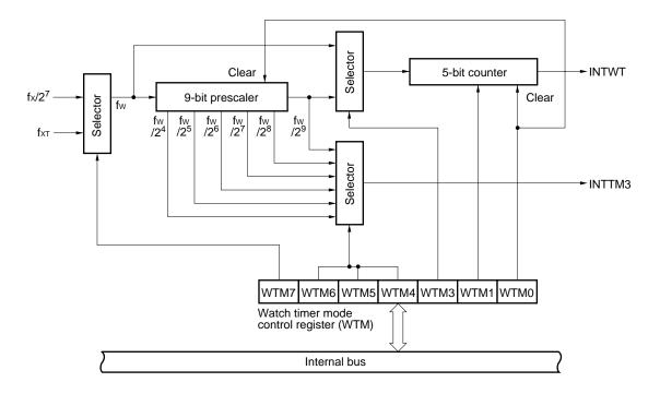
Remark fx: Main system clock oscillation frequency
