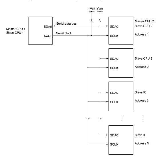
Figure 19-1. Serial Bus Configuration Example in I<sup>2</sup>C Bus Mode
