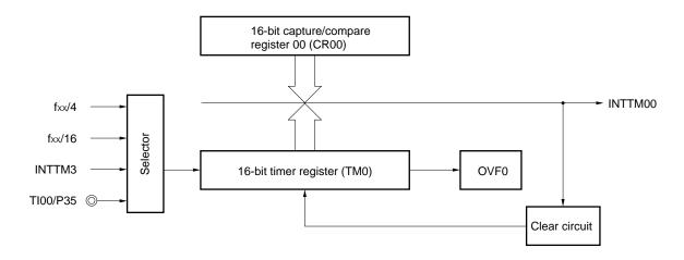
Figure 8-8. Timing of Interval Timer Operation
