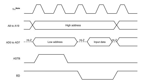
Figure 24-14. Read/Write Timing by Address Wait Function (3/3)
