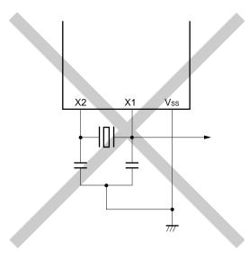
**Remark** When using a subsystem clock, replace X1 and X2 with XT1 and XT2, respectively. Also, insert resistors in series on the XT2 side.
