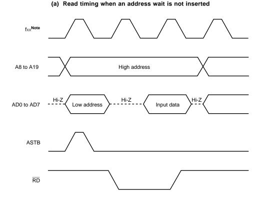
**Note** fxx: Main system clock frequency. This signal is only in the  $\mu$ PD784218.
