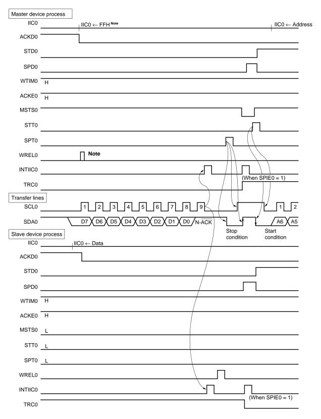
**Note** Release the slave wait by either IIC0  $\leftarrow$  FFH or setting WREL0.
