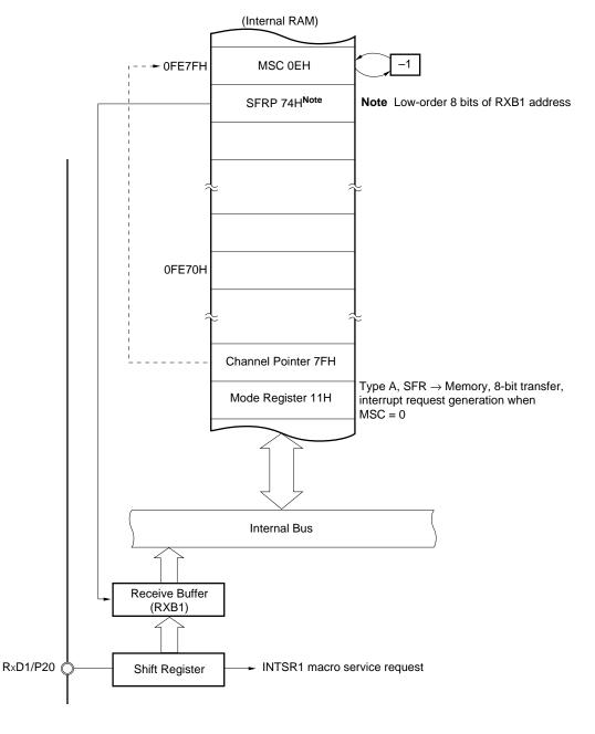
Figure 23-25. Asynchronous Serial Reception
