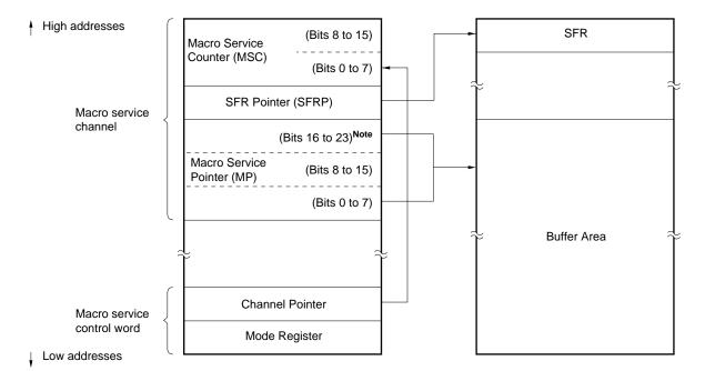
Figure 23-27. Type B Macro Service Channel
