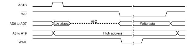
Figure 24-9. Read Modify Write Timing for External Memory in Multiplexed Bus Mode
