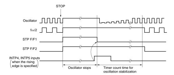
Figure 25-8. Example of Releasing STOP Mode by INTP4 and INTP5 Inputs
