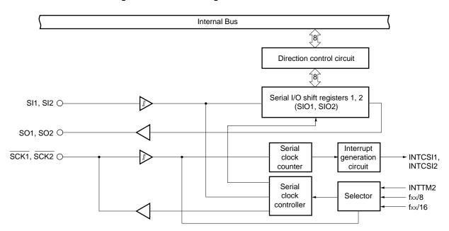
Figure 17-12. Block Diagram in 3-Wire Serial I/O Mode
