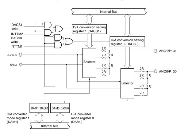
Figure 15-1. D/A Converter Block Diagram
