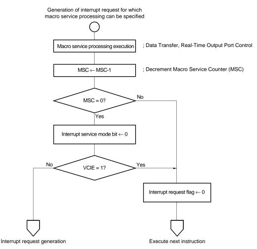
The macro service type and transfer direction are determined by the value set in the macro service control word mode register. Transfer processing is then performed using the macro service channel specified by the channel pointer according to the macro service type.
