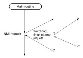
Figure 23-10. Non-Maskable Interrupt Request Acknowledgment Operations (2/2)
