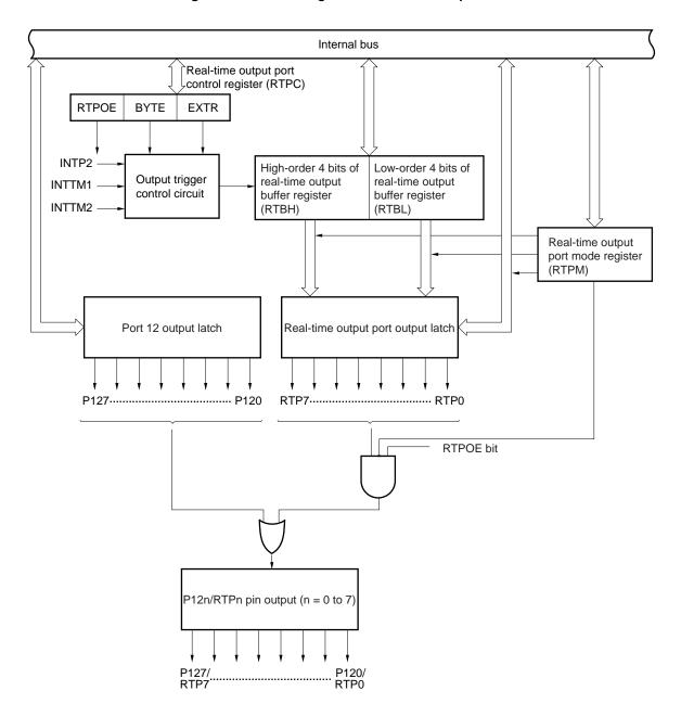
Figure 6-1. Block Diagram of Real-time Output Port
