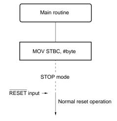
Figure 25-6. Operation after STOP Mode Release (2/2)
