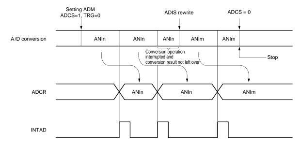
Figure 14-7. A/D Conversion Operation by Software Start
