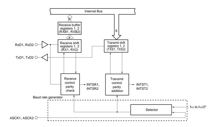
Figure 17-2. Block Diagram in Asynchronous Serial Interface Mode
