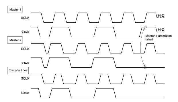
Figure 19-14. Example of Arbitration Timing
