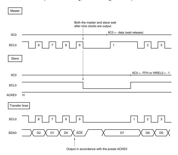
**Remark** ACKE0 : Bit 2 in  $I^2C$  bus control register (IICC0)
