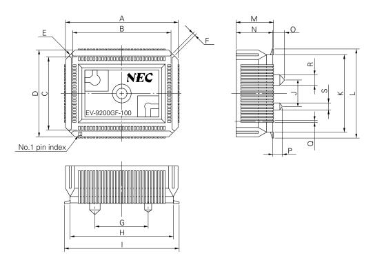
Figure B-2. Package Drawing of EV-9200GF-100 (Reference)
