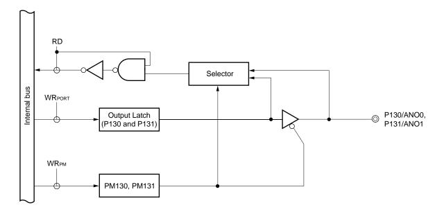
PM : Port mode register RD : Port 13 read signal WR : Port 13 write signal
