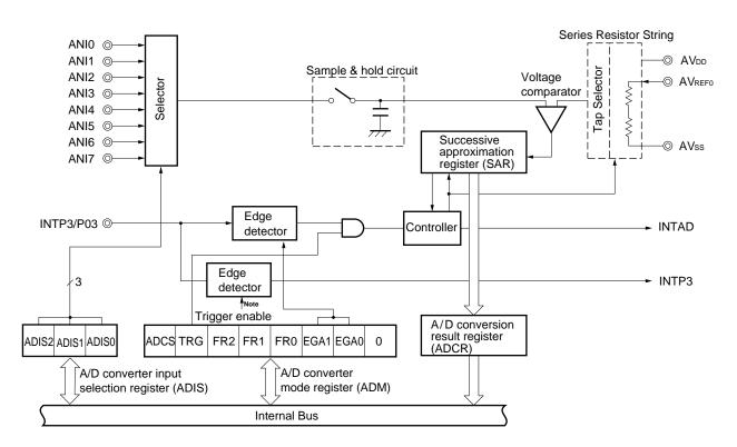
Figure 14-1. A/D Converter Block Diagram
