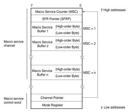
Macro service buffer address = (channel pointer) - (macro service counter)  $\times$  2 - 1
