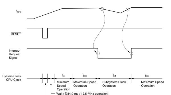
Figure 4-10. System Clock and CPU Clock Switching
