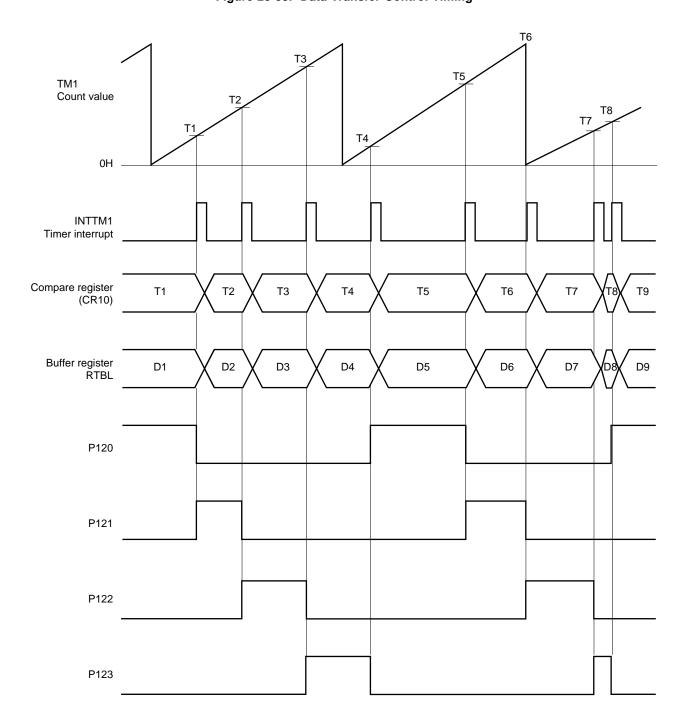
Figure 23-33. Data Transfer Control Timing
