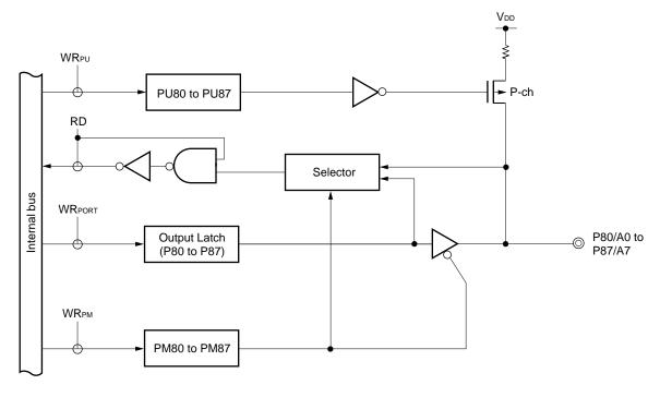
PU: Pull-up resistor option register
