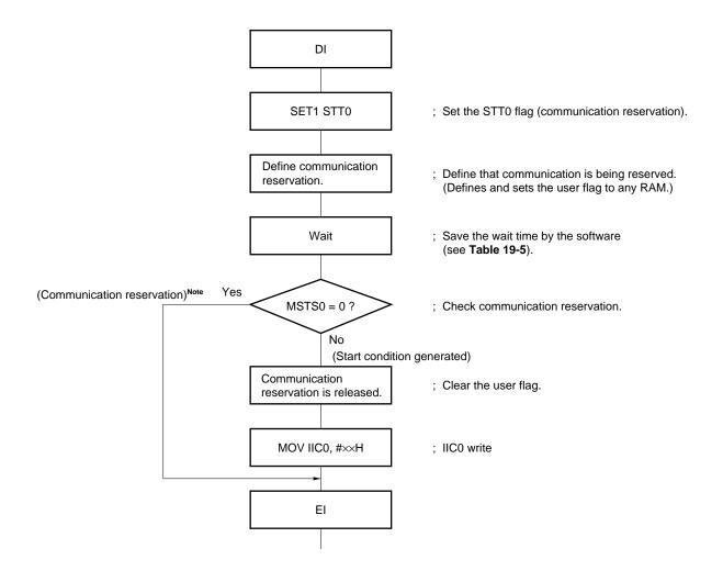
**Note** When the communication is being reserved, the serial shift register (IIC0) is written by the stop condition interrupt.
