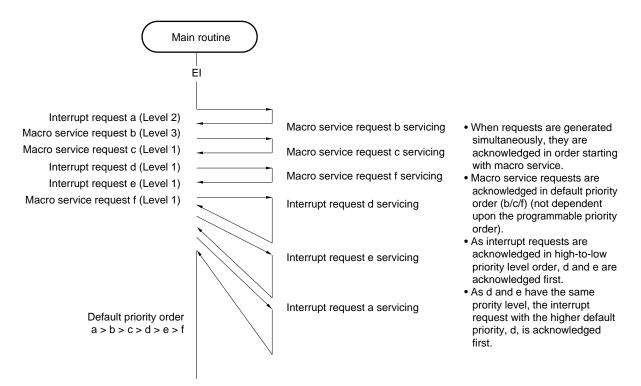
Figure 23-15. Examples of Servicing of Simultaneously Generated Interrupts
