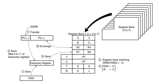
Figure 23-8. Context Switching Operation by Execution of BRKCS Instruction
