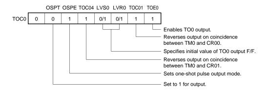
**Remark** 0/1: When these bits are reset to 0 or set to 1, the other functions can be used along with the one-shot pulse output function. For details, refer to **Figures 8-2**, **8-3**, and **8-4**.
