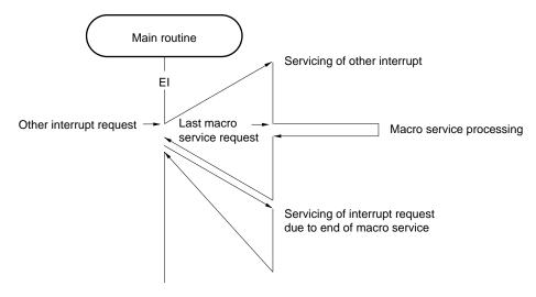
If the last macro service is performed when the interrupt due to the end of macro service cannot be acknowledged while other interrupt servicing is being executed, etc., that interrupt is held pending until it can be acknowledged.
