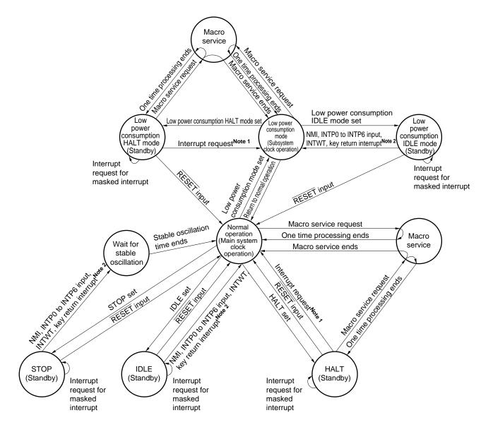
Figure 25-1. Standby Function State Transitions
