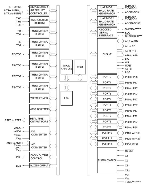
**Notes 1.** The SDA0 and SCL0 pins are provided only for the  $\mu$ PD784218Y Subseries.
