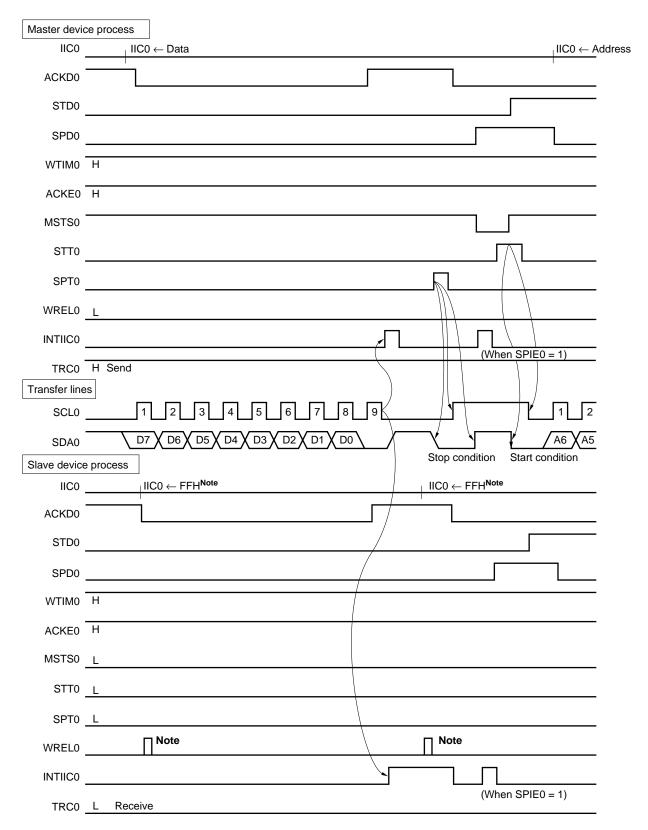
$\textbf{Note} \ \ \text{Release the slave wait by either IIC0} \leftarrow \text{FFH or setting WREL0}.$
