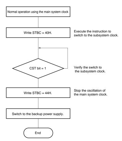
Figure 25-11. Flow for Setting Subsystem Clock Operation
