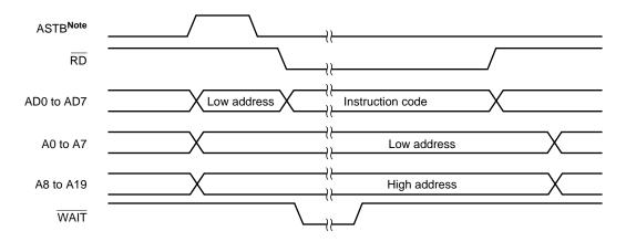
Figure 24-11. Read Timing for External Memory in Separate Bus Mode
