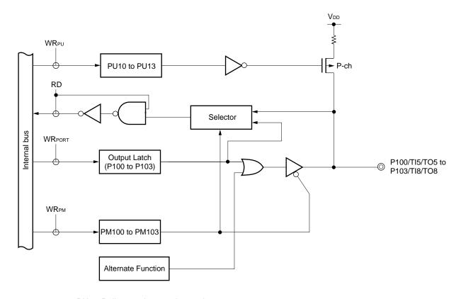
PU: Pull-up resistor option register
