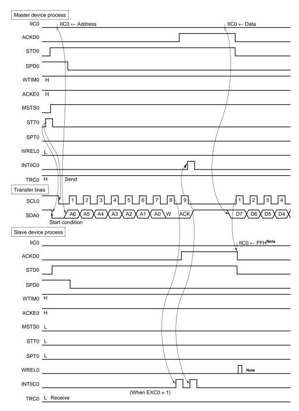
**Note** Release the slave wait by either IIC0  $\leftarrow$  FFH or setting WREL0.
