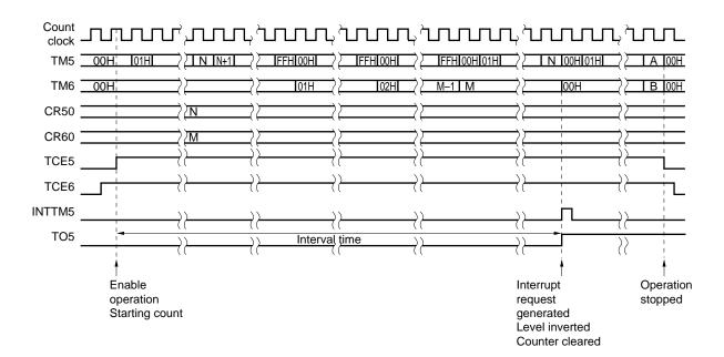
Figure 10-10. Cascade Connection Mode with 16-Bit Resolution
