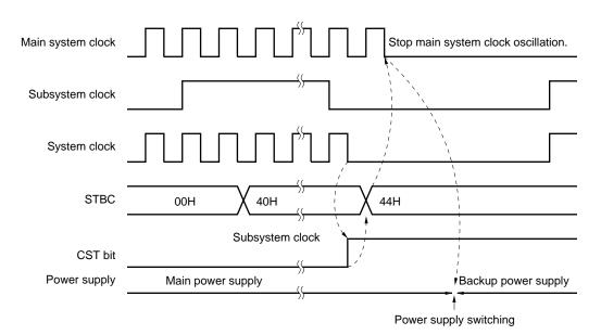
Figure 25-12. Setting Timing for Subsystem Clock Operation
