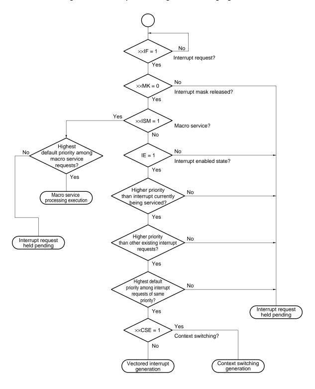
Figure 23-11. Interrupt Acknowledgment Processing Algorithm
