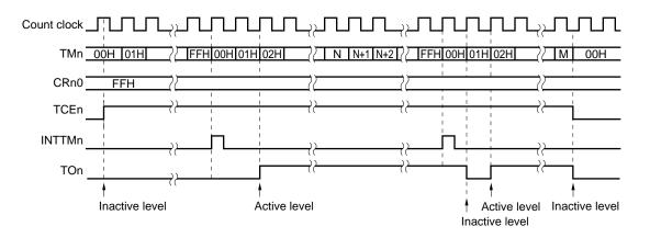
Figure 11-9. Timing of Operation Based on CRn0 Transitions
