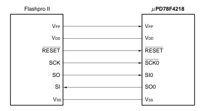
Figure 28-3. Flashpro II Connection in UART Method (when using UART1)
