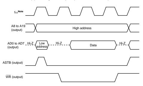
Figure 24-16. Write Timing by Access Wait Function (2/2)
