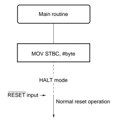
Figure 25-5. Operation after HALT Mode Release (2/4)
