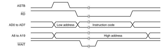
Figure 24-7. Read Timing for External Memory in Multiplexed Bus Mode
