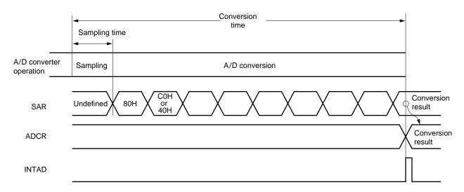
Figure 14-4. Basic Operations of A/D Converter
