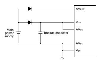
Figure 14-11. Handling of AVDD Pin
