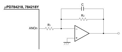
• The input impedance of the buffer amp is  $R_1$ .
